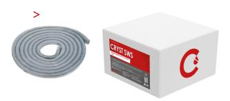
CRYST SWS® is a swellable bentonite water stop tape for sealing vertical and horizontal structural joints, which are exposed constantly or temporarily to water. CRYST SWS® Swelling Tape is designed for use in non-movement joints of concrete. In contact with water, the reaction of the tape is activated and the tape starts swelling. Due to the swelling pressure in the construction joint, leads to penetration into cracks, joints, cracks, cavities, and seals the area.
